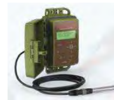
Figure 114 : SM4 de Wildlife Acoustics (source : CALIDRIS, 2020)
